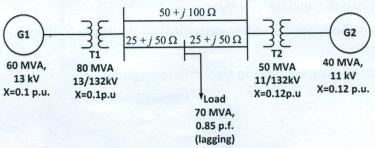
13. a) For the network shown in the Figure below, Calculate the  $Z_{BUS}$  matrix. The impedance values are as follows:
